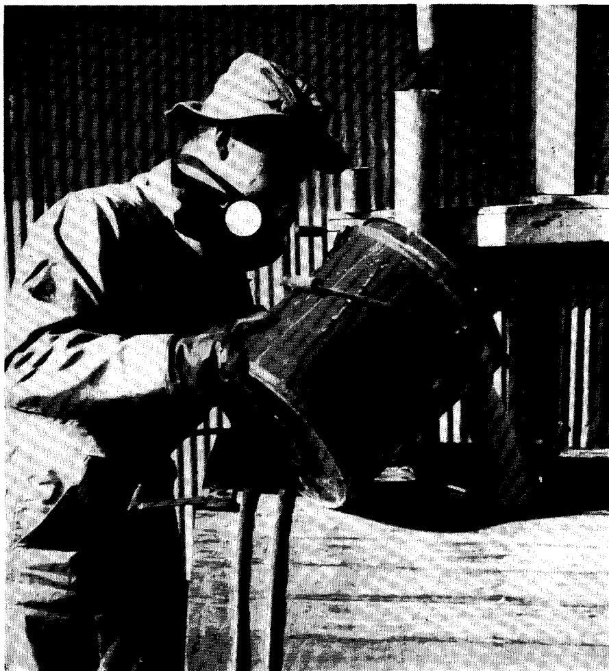
A respirator and gloves should be worn when dangerous chemicals are handled
