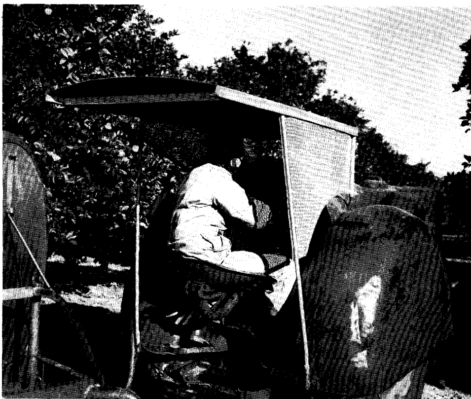
Removable canopies on tractors help to minimize the spray drift hazard
